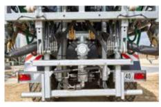
Fliegl SKATE 210 with pendulum frame for better slope compensation (only on SKATE 210/240)
