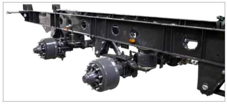
Special frame construction made from fine-grain steel
