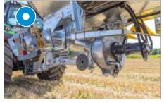
For vacuum tank: turbo filler positioned centrally under tank – for suction on either side
