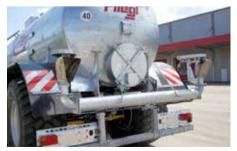
Double pendulum spreader, hydraulic
