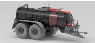
Residual emptying takes place once the slurry volume in the rear chamber has dropped to a level that allows air to enter the front chamber via the separating wall.
