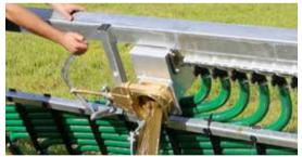
Trap box for foreign objects, emptied mechanically or hydraulically
