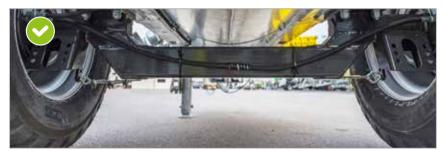
Cranked axle on 5000 to 8600 I models Low centre of gravity ensures optimum handling on slopes
