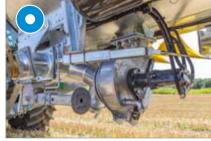
For vacuum tank: turbo filler positioned centrally under tank for suction on either side
