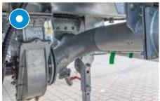
Hydraulic turbo filler, centrally under tank
