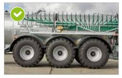
Individual wheel arches in combination with hydr. suspension
