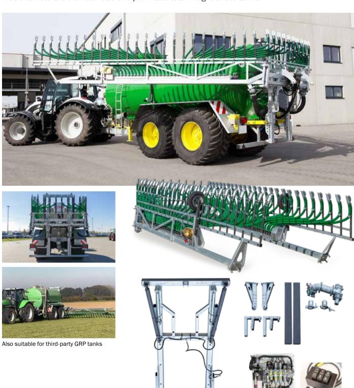
Scope of delivery: pre-assembled trailing shoe spreader, control panel and control block, H-frame, transport lock, T-piece with flexible hoses for the slurry feed
