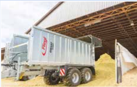
Pushing off, not tipping - so no problems even in low buildings.
