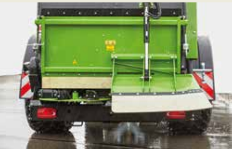
Edge spreading device Available as single attachment for left or right, or for both sides.
