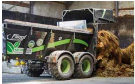
As an option, the ADS can be retrofitted with an 800mm large-area back wall for use as a transport trailer
