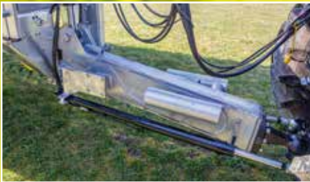
Optional: hydraulic forced steering
