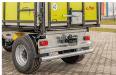
Lighting carrier with automatic trailer coupling and grain slide
