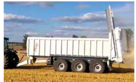
Wide-spreading back wall
