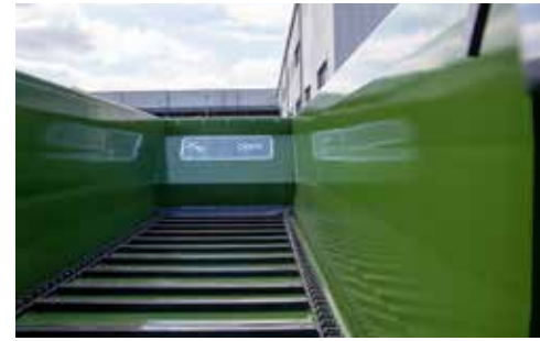
KDS 260: body made from fine-grain steel
