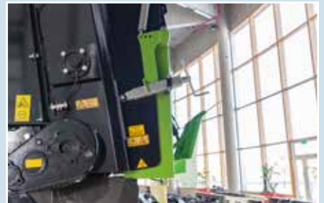
Drive train of the horizontal rollers. Overload protection via ratchet clutch in drive shaft to tractor.
