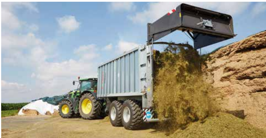
Dosing roller with 3 horizontal milling drums
