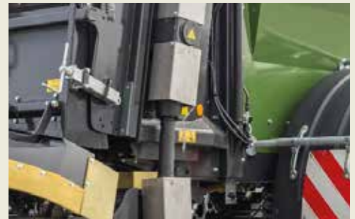
Milling drum drive above drive shaft
