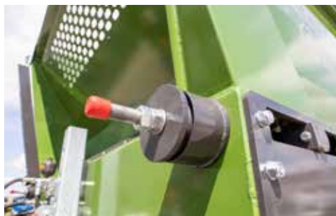
Mechanical chain tensioning
