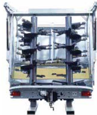
Milling drums with throwing vanes
