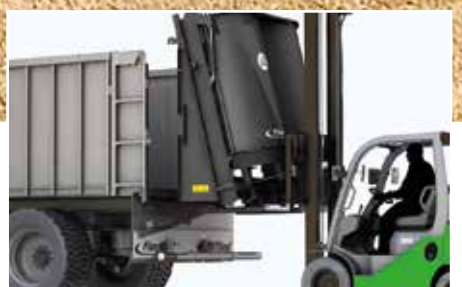
With a stacker truck, all spreading units can be installed easily within about 20 minutes.
