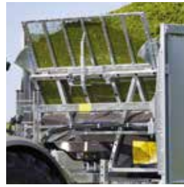
New push-off wall „Insight“ made of shatter resistant material
