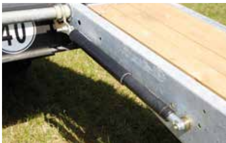
Drive-on ramps as standard with spring jack, and hydraulically operated as option
