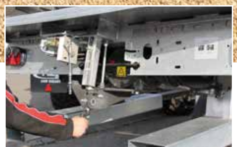
Push-off speed is adapted automatically by the automatic feed control
