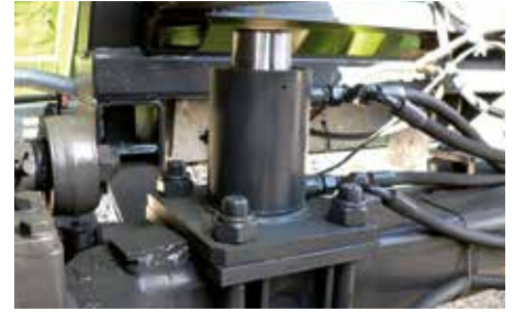
Optional: hydraulic support at the axle
