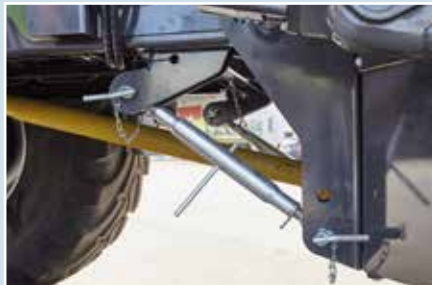
Drive train of the horizontal rollers. Overload protection via ratchet clutch in drive shaft to tractor.
