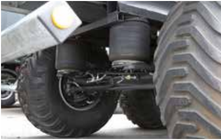
Optional: air suspension with automatic lowering when tipping
