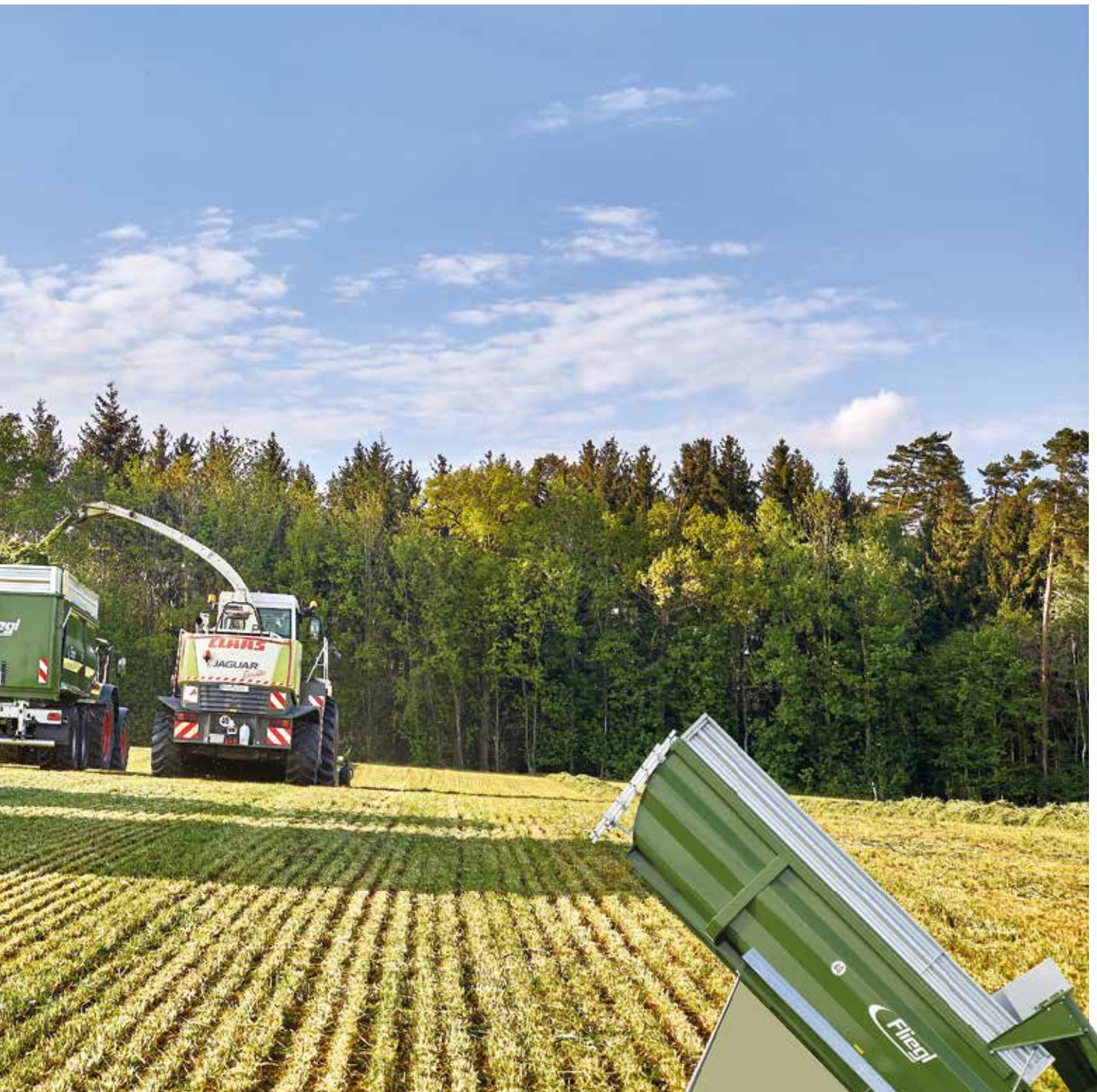
Tandem TMK 269 Profi with body length 6.90 m and tilt angle about 55°
