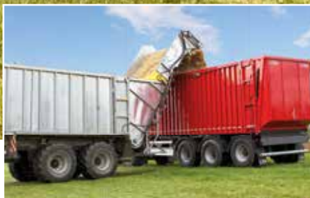
“MobilFast” overloading belt (up to 30m 3 /min)
