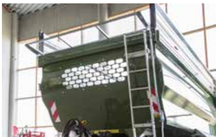
Mechanically folding protective grating
