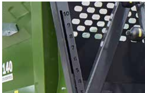
The sliding gate opening scale on the front shows the opening position of the sliding gate.
