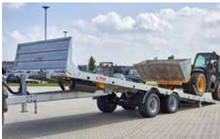
From TPA 200 on: Hydraulic tipping drawbar
