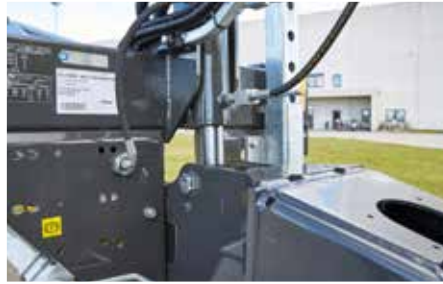
Hydraulic drawbar suspension
