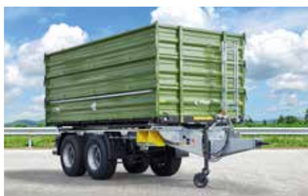
TDK 160 with 1800 mm body (3 x 600 mm tailgate)
