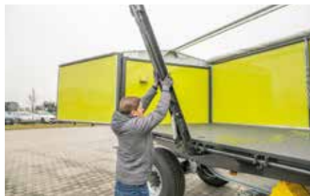
Removable centre stanchion for effortless loading and unloading
