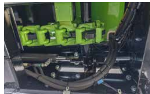
Hydraulic chain tensioning
