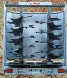
Milling drums with slingers
