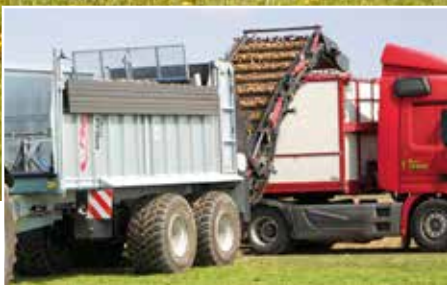
“PomOver” potato overloading belt
