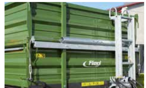
Optional: tailgate tension spring in heavy-duty version
