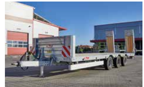
The TPA 370 Bulkhead 800 mm as standard Folding drive-on ramps
