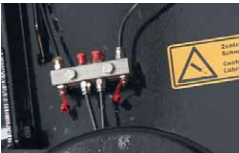
Central lubrication point
