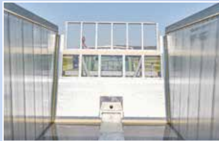
Sealing strips: Special polyurethane strips arranged at a 45° angle seal the loading area perfectly.
