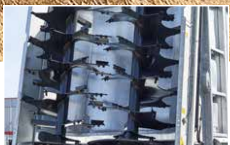
The milling drums break up the spreading material for uniform results.
